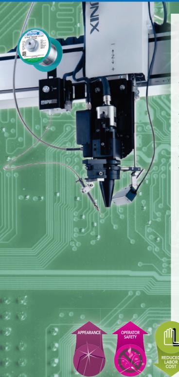
Both PCB and component size has become increasingly smaller in recent years creating a strong demand for ultrafine wire (diameter ≤0.20mm) technology. With the maturity in laser soldering technology, ultrafine cored wire maximizes the potential of fine wire application in high density boards.
